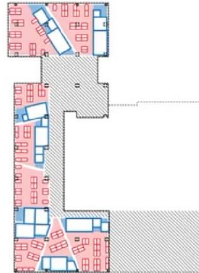
⑥ Automated "test fit" generates amenity rooms from space matrix and desk layout.
